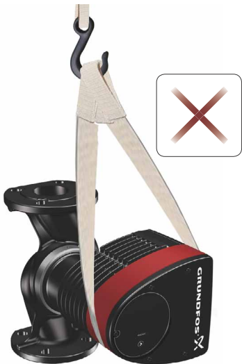
Fig. 6 Incorrect lifting of pump
