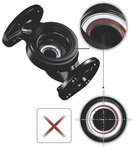
Fig. 12 Incorrectly centred sealing system
